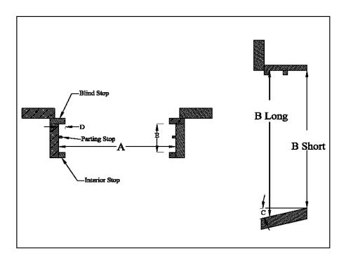
**Note on window stools**: To properly hide the bottom sash weatherstripping of the insert window the stool height must be at least 7/8" off the sill. If the exiting stool is less than 7/8" a quarterround or other profile trim piece can be added to the top of the stool after installation.
